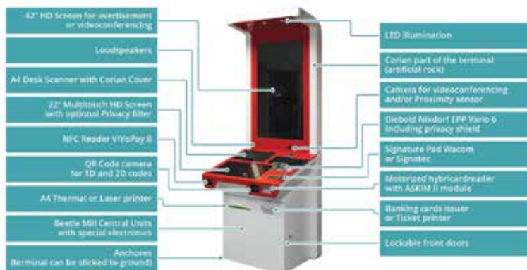
Fig. 31. Main components of the VTM.iQ computer appliance.
